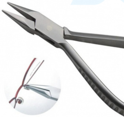
Flat Semicircular Snipe Nose Pliers AI-01-128 Semi-circular with flat milled jaws for better hold, small tips make it easy to reach into tighter areas for adjust angle and shape of pad arms. Also for shaping and bracing. Tapers to a fine point. Length: approx. 150 mm Jaws Tip: Diameter 1.5 mm Weight: approx. 102.5 g
