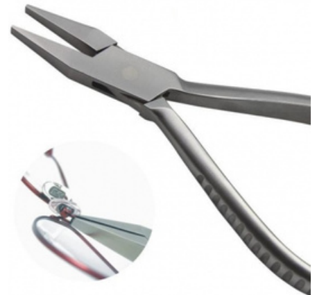
Flat Nose Pliers 4.5mm AI-01-127 Flat milled jaws with 4.5mm width for better hold. Used for general purposes, particularly useful for adjust of pad arms & holding temples on thin metal frames. Length: approx. 150 mm Jaws Width: 4.5 mm x 1.2mmH Weight: approx. 115.5 g
